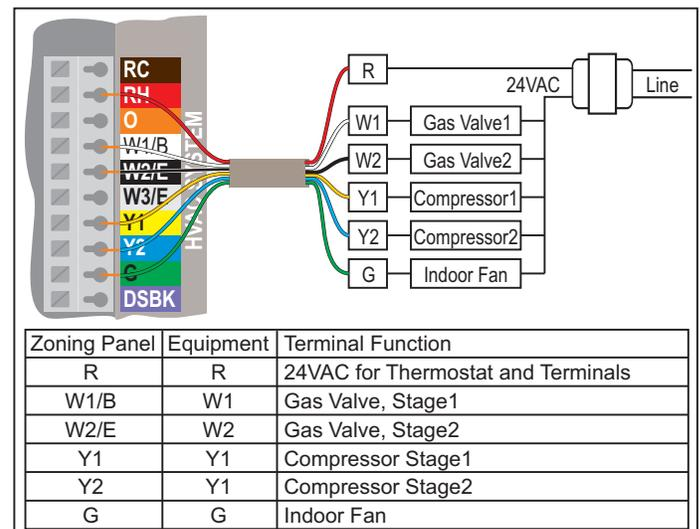
Figure 24. Wiring a Gas/Electric system with 2 heating and 2 cooling stages.
