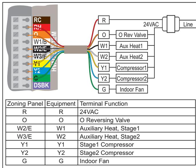
Figure 25. Wiring a Heat Pump system with a 2-stage compressor and 2 auxiliary heating stages.
