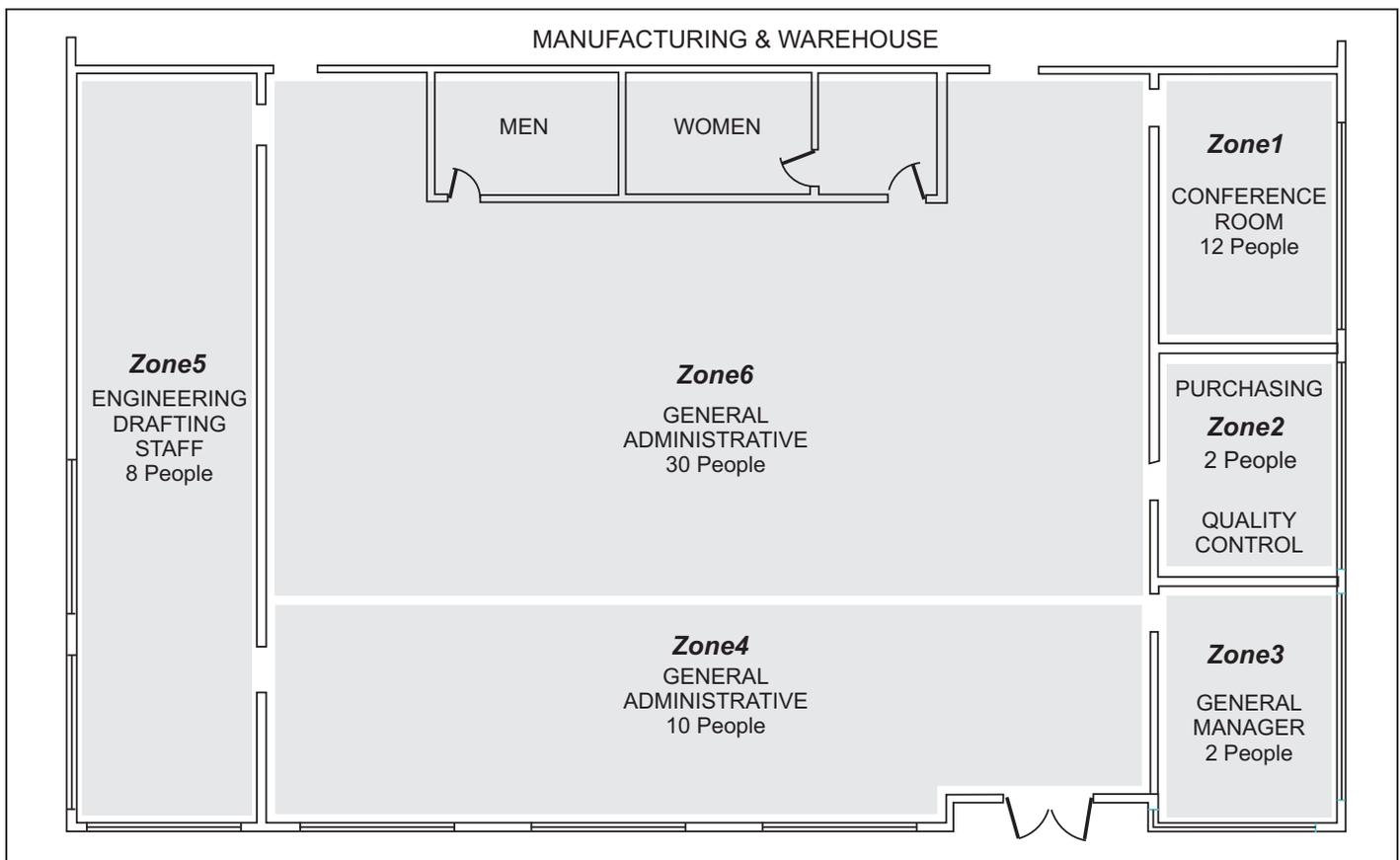
Figure 4. Zoning plan for manufacturing facility.
