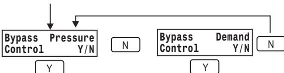
Press Yes to select using the Duct Pressure sensor to control Bypass using the non-calling zone dampers and continue to set the H2O Bypass Limit.
