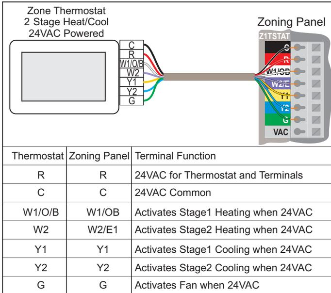
Figure 14. Wiring 2-stage, Heat/Cool, 24VAC zone thermostat
