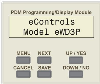
When accessing the Installer menu, the PDM will read a description of the panel and only those options compatible with the panel can be set.
