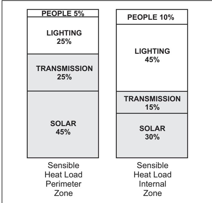
Figure 3. Sensible heat load for perimeter and internal zones.
