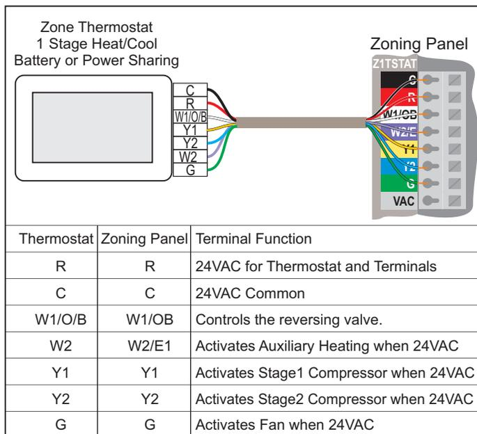
Figure 15. Wiring 1-stage, Heat/Cool, battery powered or power sharing zone thermostat.
