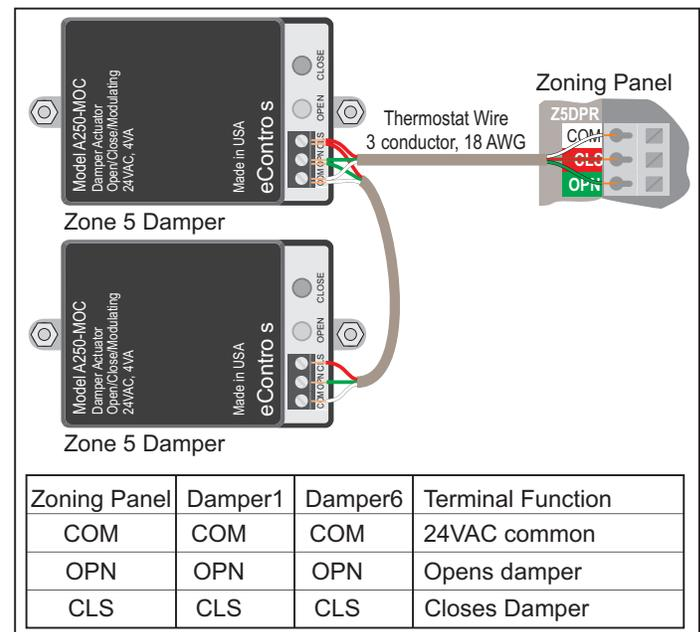
Figure 11. Wiring CRDA250 actuators when multiple dampers are used to form a zone.
