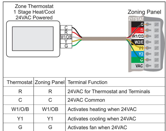
Figure 13. Wiring 1-stage, Heat/Cool, 24VAC zone thermostat.
