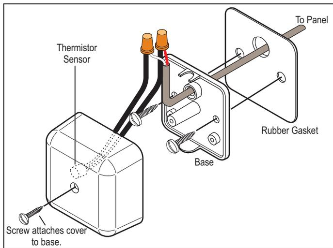
Figure 19. Outdoor temperature sensor wiring.
