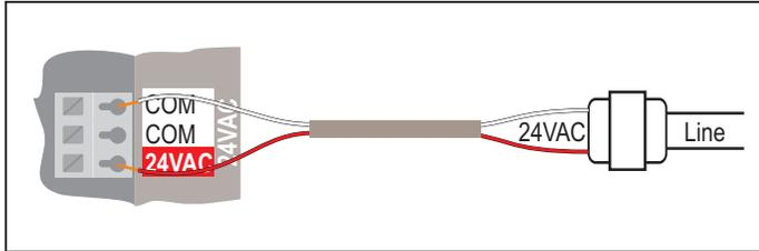
Figure 8. 24VAC power wiring for panel and dampers.
