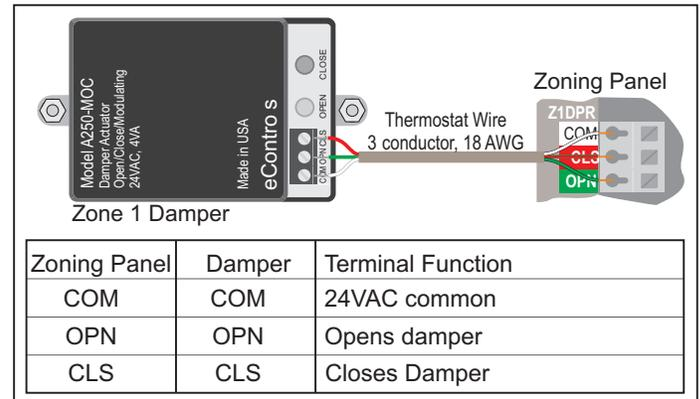
Figure 10. Wiring CRDA250 actuator.
