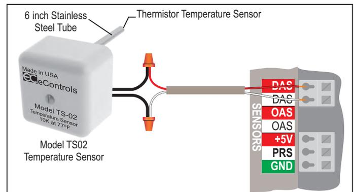
Figure 20. Discharge Air temperature sensor connection.
