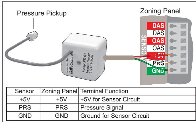
Figure 22. Duct Pressure sensor connection.
