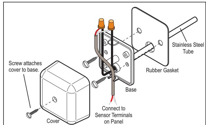
Figure 21. Discharge Air temperature sensor wiring.
