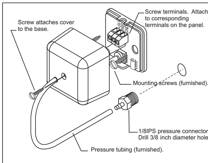
Figure 23. Duct Pressure installation.
