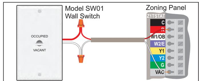
Figure 16. Wall switch used to control Vacant mode.
