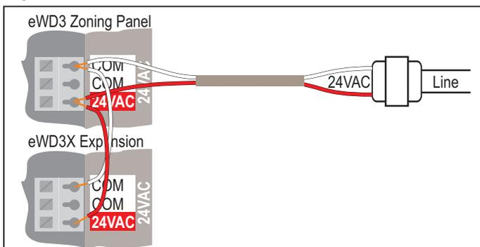
Figure 9. One transformer powering eWD3P and eWD3X.
