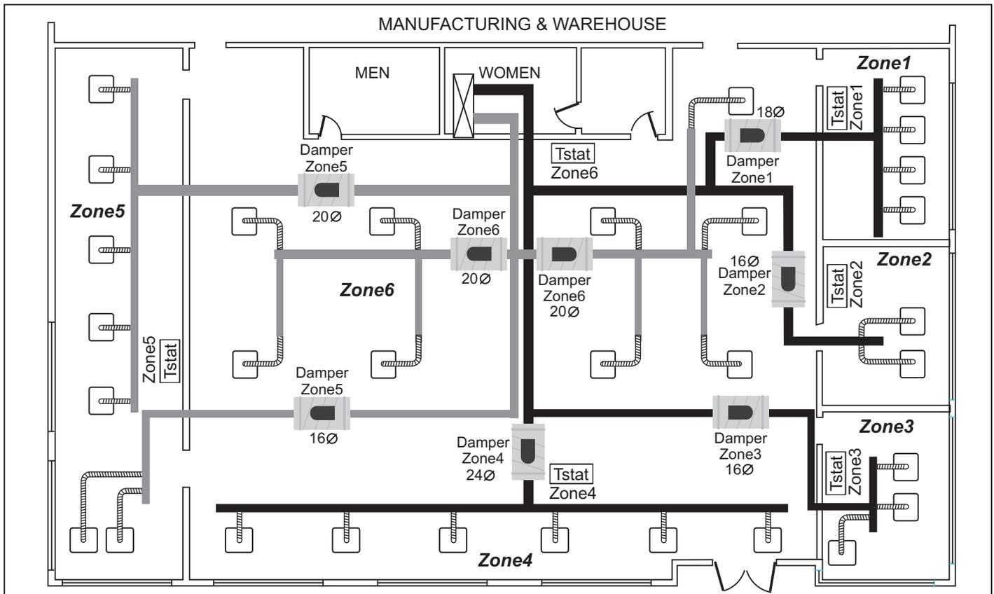
Figure 6. Damper and thermostat placement.
