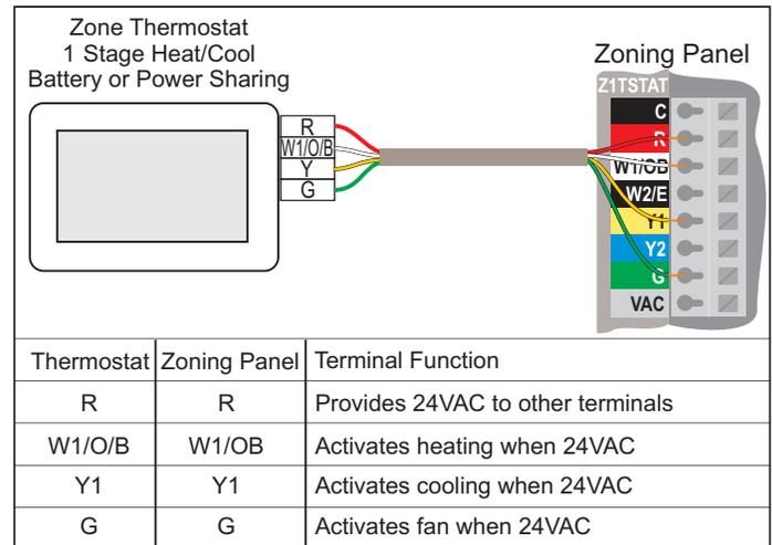
Figure 12. Wiring 1-stage, Heat/Cool, battery powered or power robbing zone thermostat.
