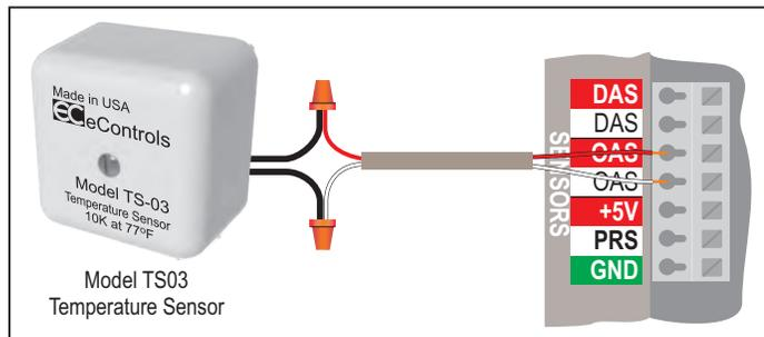
Figure 18. Outdoor temperature sensor connection.
