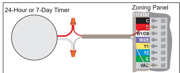
Figure 17. Timer used to control Vacant mode.
