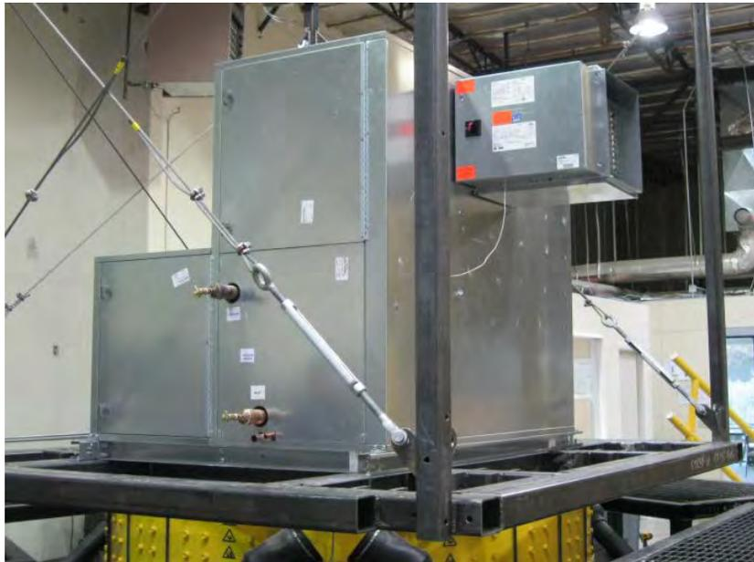
Unit was rigid base mounted to the shake table interface fixture with 1/2-inch threaded rod at each of the four corners.
