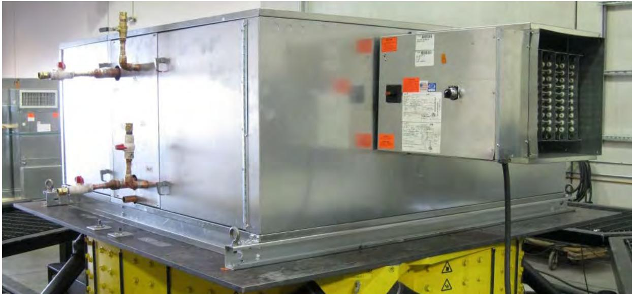
Unit was rigid base mounted to the shake table interface fixture four 1/2-inch diameter Grade 5 bolts, one on each corner of the unit, using the manufacturer-provided mounting tabs.
