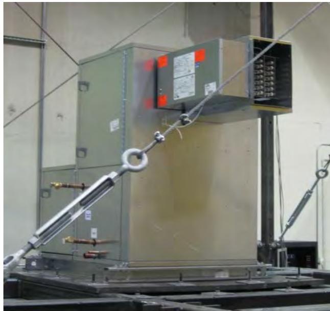
Unit was rigid base mounted to the shake table interface fixture with 1/2-inch threaded rod at each of the four corners.
