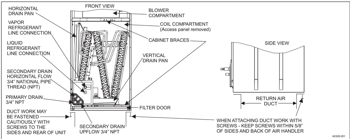
**FIGURE 1:** Return Air Duct Attachment & Component Location
