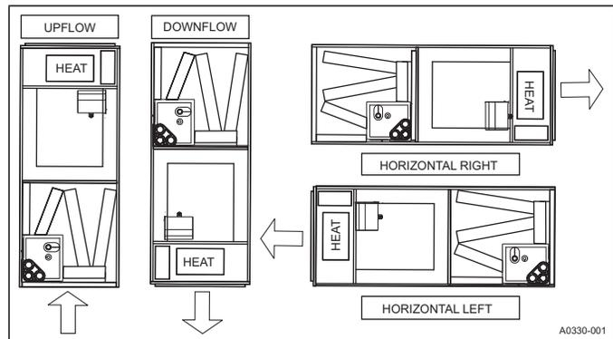
FIGURE 4: Typical Installation
