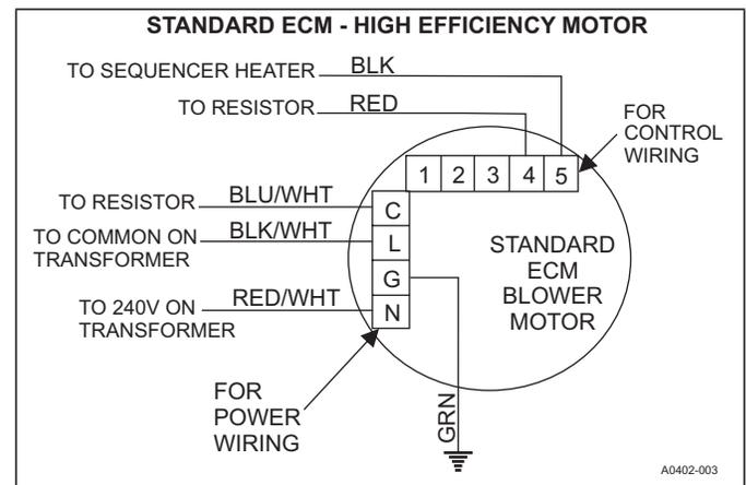
FIGURE 17: Blower Speed Connections
