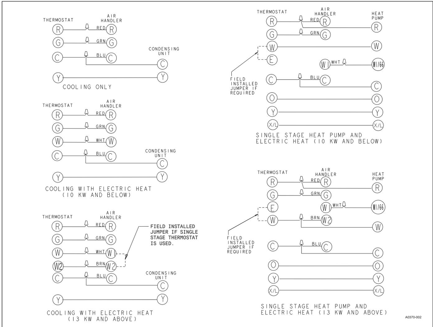
FIGURE 23: Typical Thermostat Wiring Diagram - ECM
