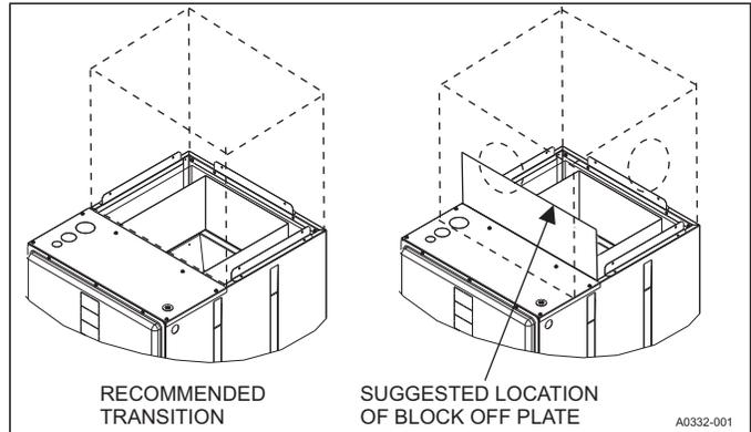
**FIGURE 8:** Duct Work Transition
