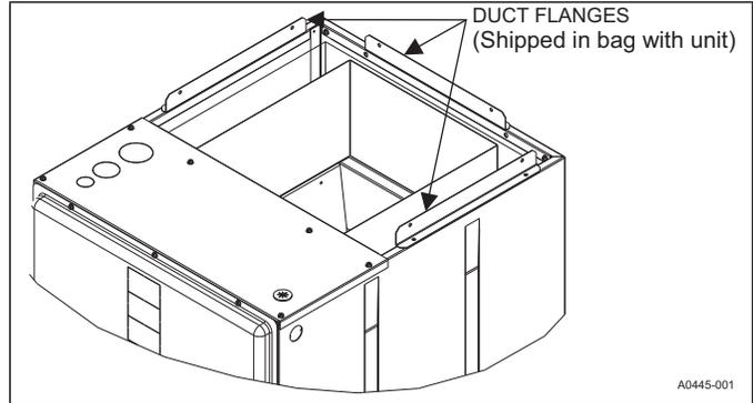
**FIGURE 7:** Duct Attachment
