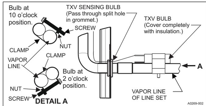
FIGURE 13: Proper Bulb Location
