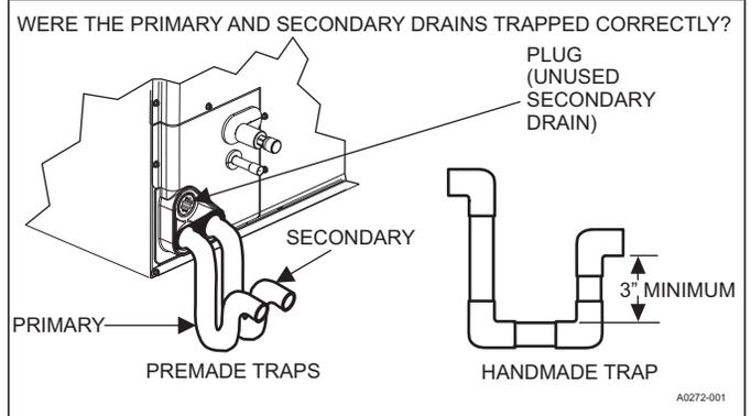
FIGURE 19: Drain Traps
