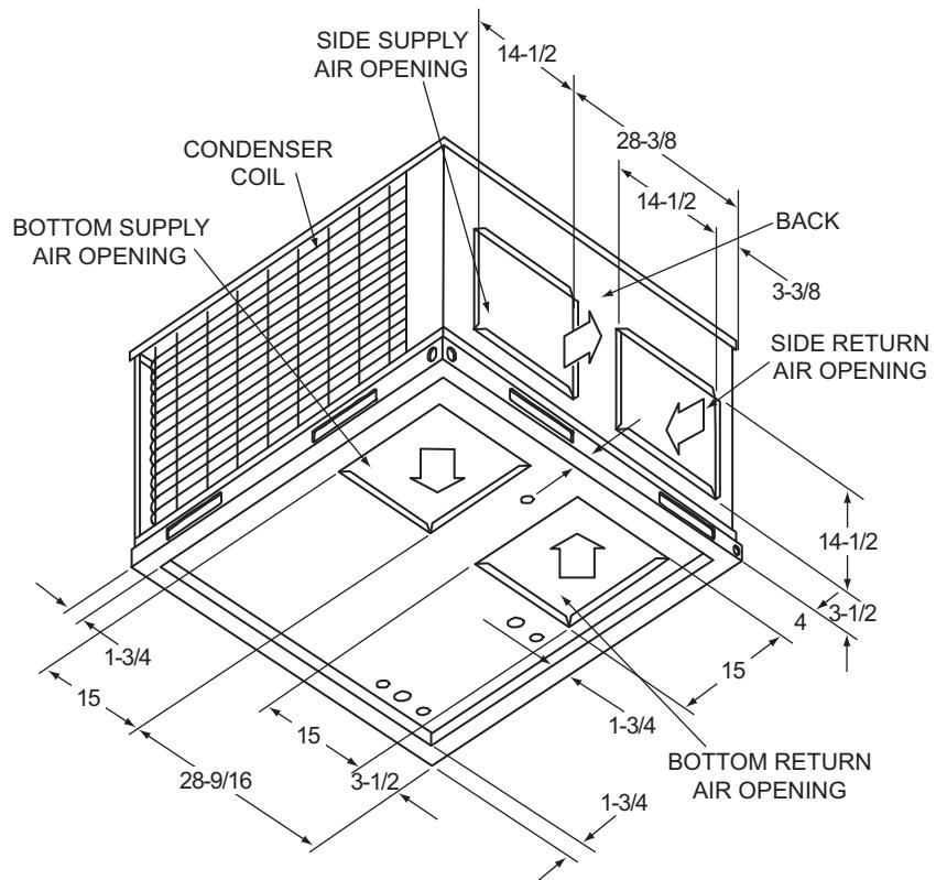
**Unit Typical Duct Applications**
