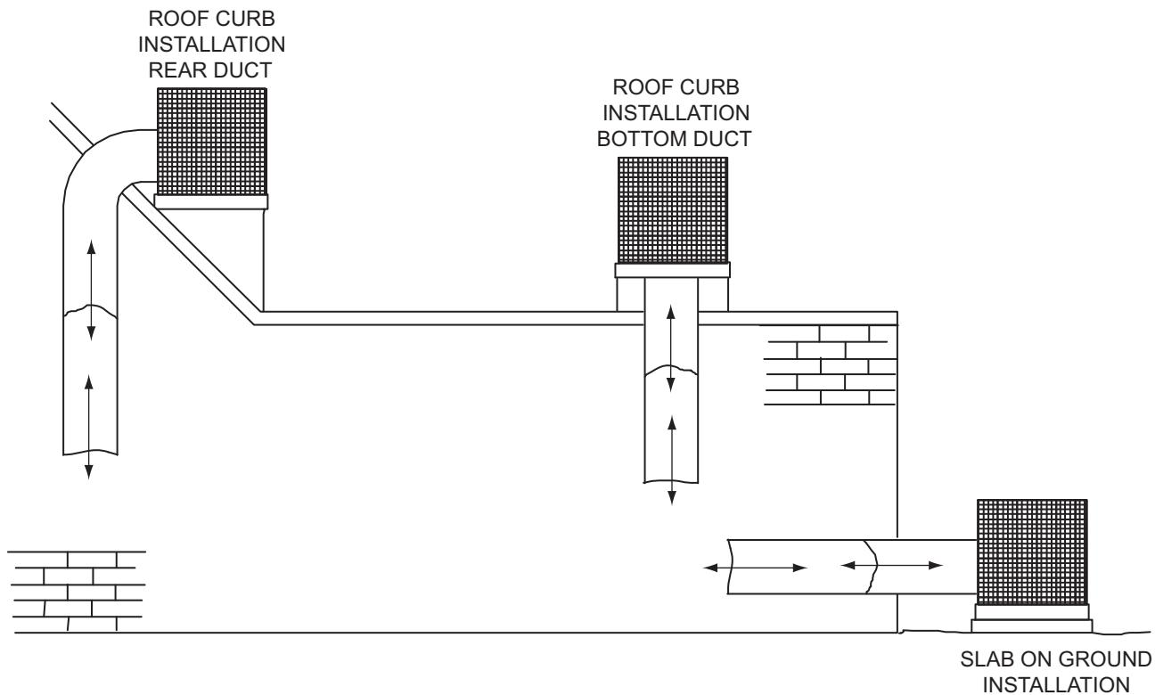
**Unit Typical Slab on Ground Installation**
