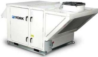
JR Series Unit | 3 – 70 Tons | Up to 18,000 CFM | AC, Gas, Water, Electric, Air Source HP, Water Source HP | Digital and VFD Scroll Compressors | Modulating Hot Gas Reheat | Energy Recovery Module | Double Wall Construction | MERV-14 Filters
