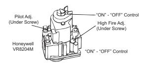
Figure 25: Typical Single Stage Gas Valves
