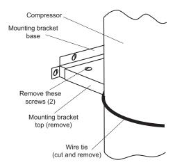
Figure 12: Compressor Restraining Bracket
