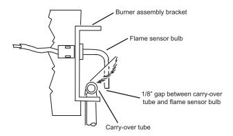
Figure 27: Proper Flame Adjustment
