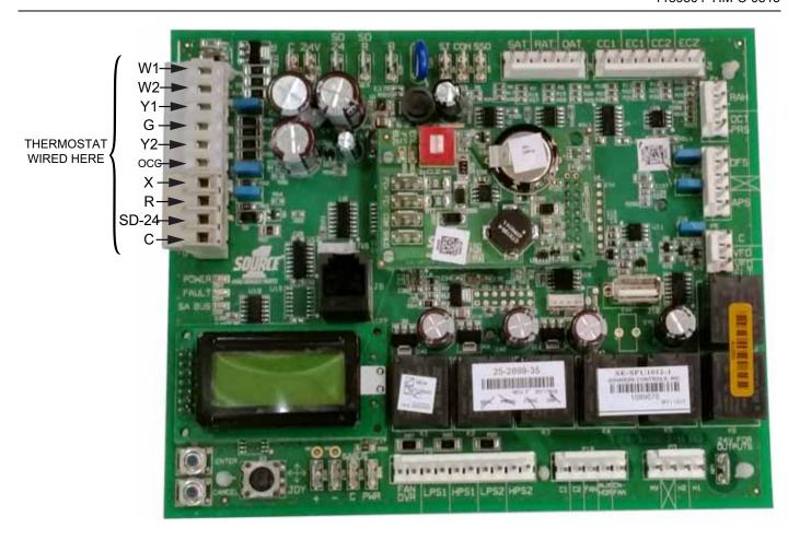
Figure 30: Unit Control Board
