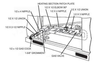
Figure 15: Side Entry Gas Piping
