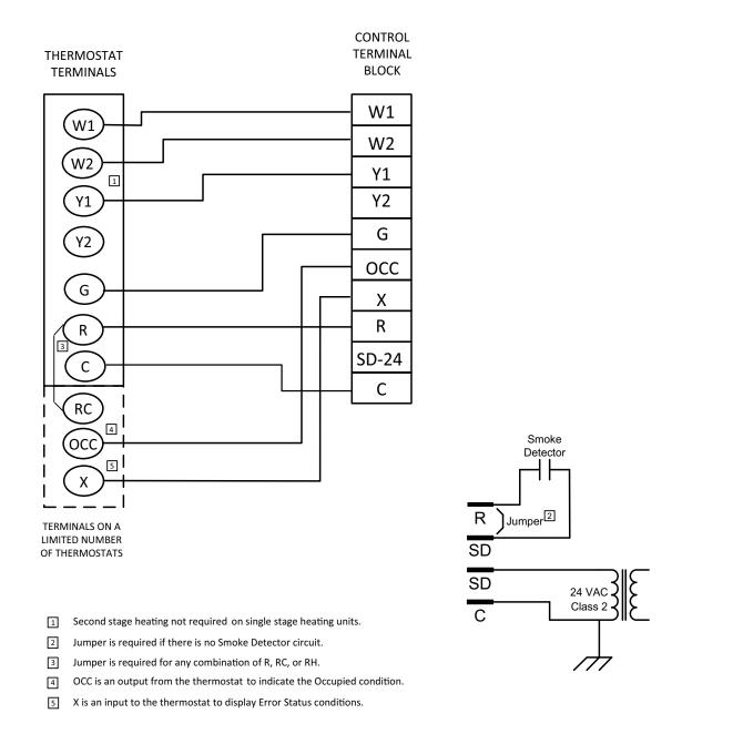
Figure 13: Typical Field Power and Simplicity Lite Control Wiring
