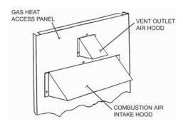
Figure 17: Vent And Combustion Air Hood
