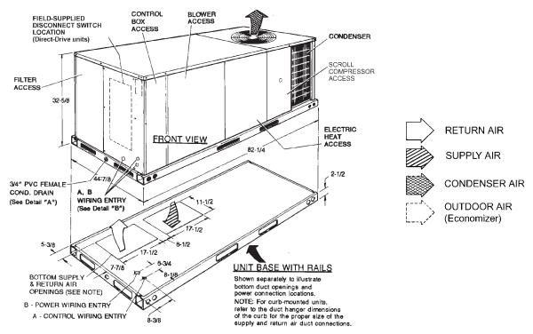
Figure 5: ZE036-060 Cooling Only/Electric Heat Front View Physical Dimensions
