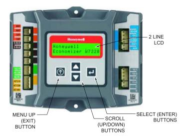
Figure 18: Economizer LCD and Keypad Layout.
