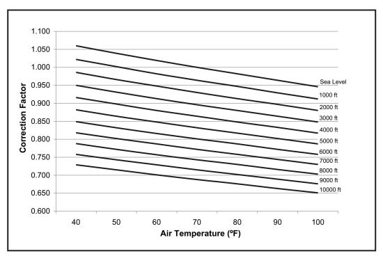
Figure 22: Altitude/Temperature Correction Factors
