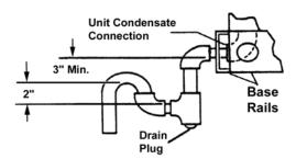
Figure 11: Condensate Drain
