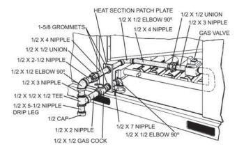
Figure 16: Bottom Entry Gas Piping
