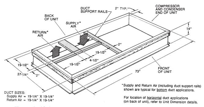
Figure 10: ZE036-060 Roof Curb
